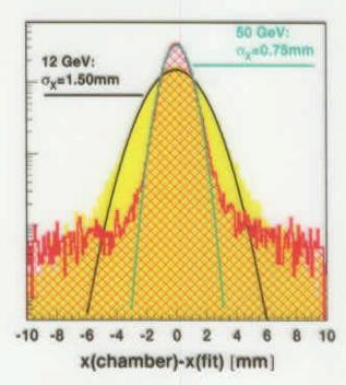
$\Rightarrow$  Position resolution  $\sigma_x \simeq 5 \text{ mm}/\sqrt{E}$  (E in GeV)
