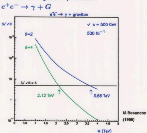
Even higher sensitivity (up to 9 TeV) can be obtained with beam polarisation (supress  $\nu\nu\gamma$ -background)
