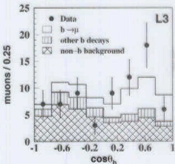
b asymmetry derived from a likelihood fit accounting for the different b semileptonic decays and background. At 189 GeV:
