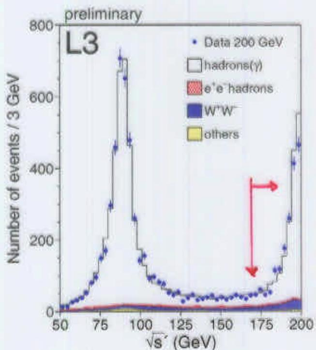
W-pair background rejected on the basis of topological information. Residual contamination  $\approx 5\text{-}15\%$
